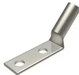
Copper Two Hole HYLUG - Long Barrel ,45 Degree Pad 350 kcmil,1/2" Bolt Hole with 1-3/4" Spacing,Tin Plated,Color: Red,Die Index: 18.
